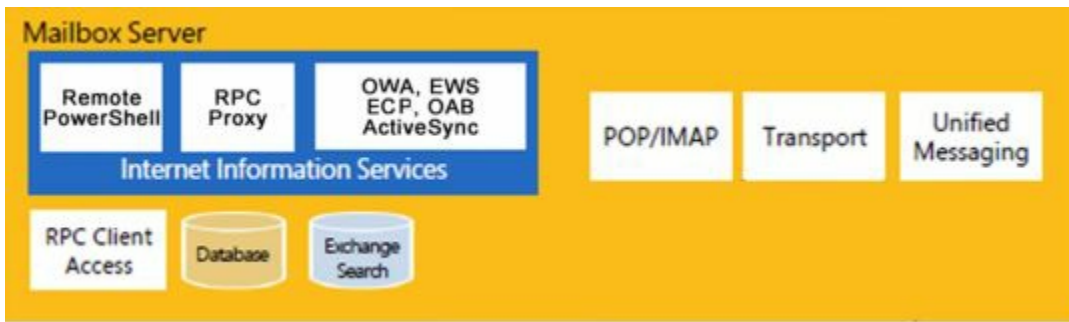
FIGURE 17-2 Connections points into Mailbox servers.
